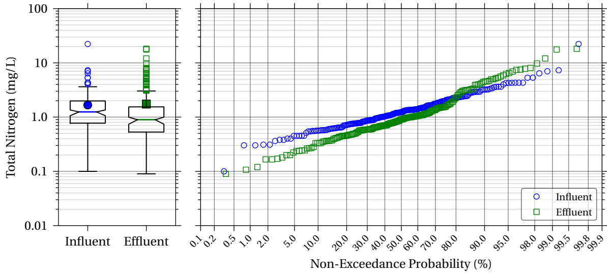
Figure 3.9: Box and Probability Plots of Total Nitrogen at Bioretention BMPs
