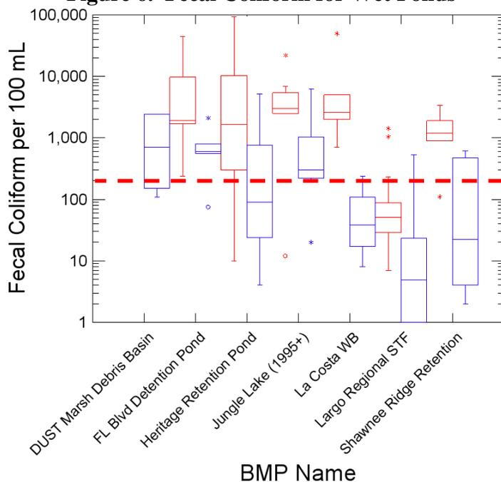
Notes: Inflow and Outflow boxes “straddle” the X axis tick marks. X axis labels restricted to 24 characters; see Attachment 1 for full BMP Names. Red dashed line provides primary recreation stream standard as a benchmark for comparison. Note: for some BMPs, only outflow data are available (e.g., DUST Marsh Debris Basin).
