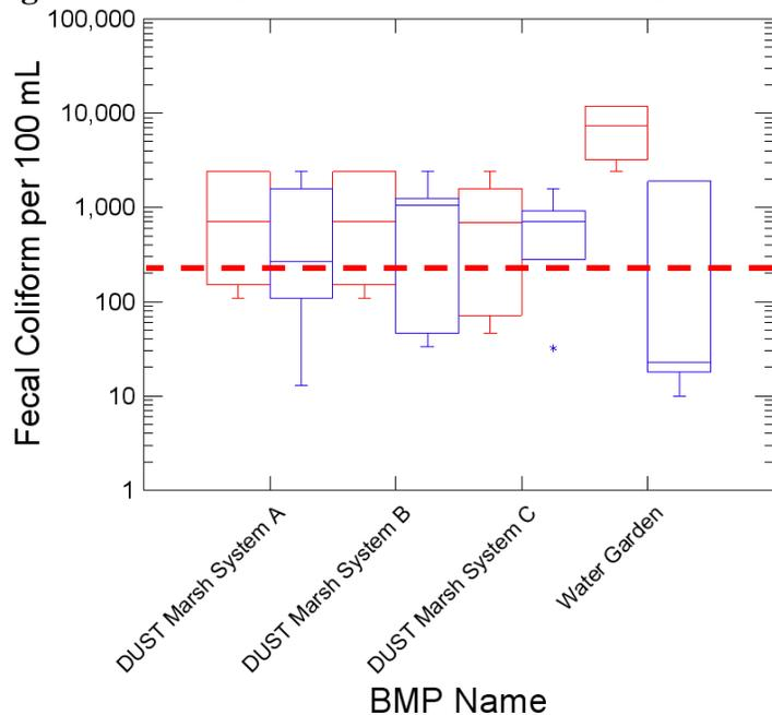
**Figure 10. Fecal Coliform for Manufactured Devices**
