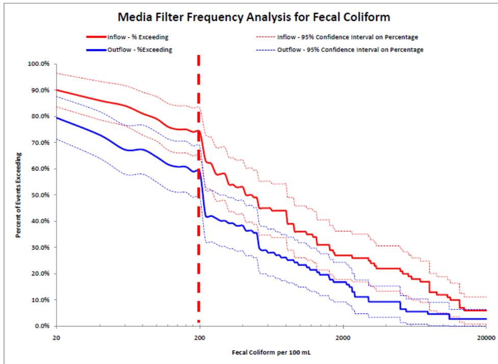
**Figure 14. Exceedance Frequency Distribution for Manufactured Devices**
