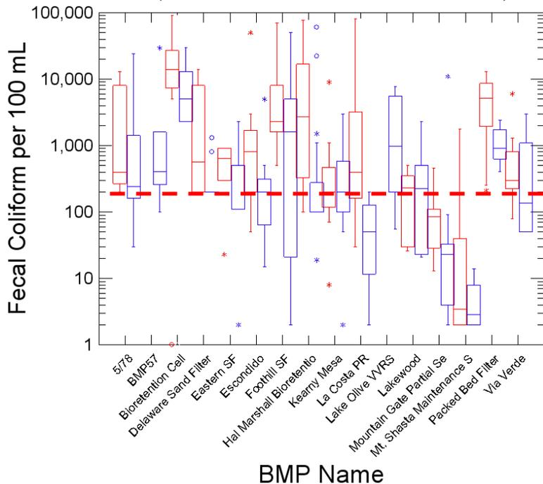
**Figure 8. Fecal Coliform for Grass Swales & Strips**
